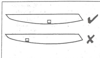
2. • If fixing directly to the hull use a polysulphide based sealing compound. However, if using screws ensure the hull thickness is greater than the screw length.
