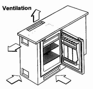
All refrigerators, regardless of the make, are heattransfer machines. They transfer the heat from inside the fridge to the outside of the fridge. If adequate ventilation is provided, the compressor will operate more efficiently, and use less power.
