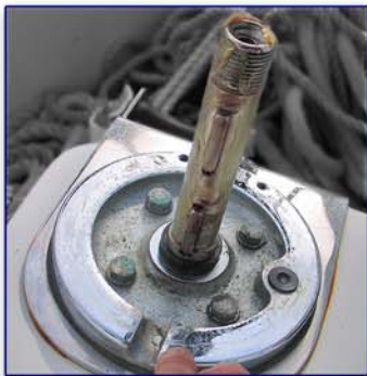
Windlass base prior to re-assembly - grease shaft & threads.
