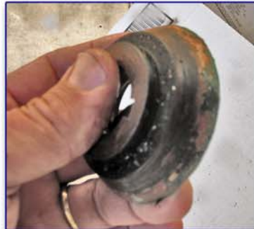
Heavy corrosion on clutch cones
