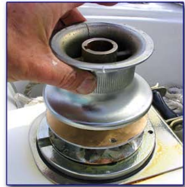
Lift drum vertically on keyed shaft
