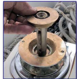
Re-assemble 3 pc brass clutch on shaft over 2 keys
