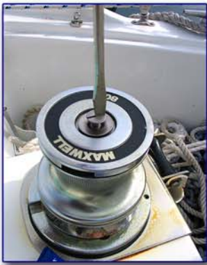
Remove Rubber Cap, screw and washer
