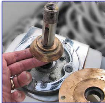
Re-assemble 3 pc brass clutch on shaft over 2 keys
